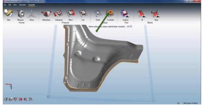
모델 Set up (Draw 방향, Holder, Drawbead)
